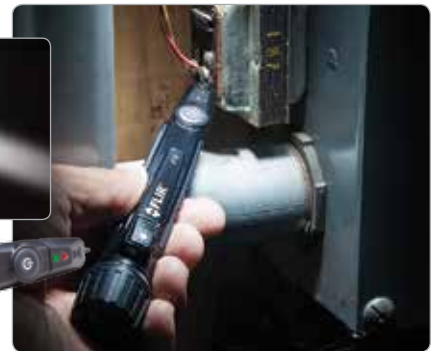
High sensitivity detects voltage in low-powered systems; visual & vibration alerts for noisy areas.
