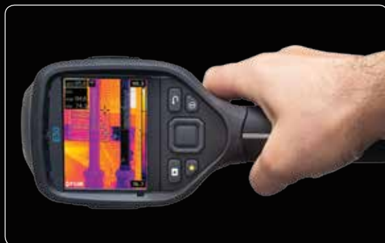
Auto-orientation keeps diagnostics overlays upright.
